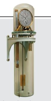
**Glass-Tank Regulator** (Germany, 1895) Sigmund Riefler made a significant improvement in timekeeping when he designed a clock that operated in a partial vacuum. Combined with a pendulum made from a metal
